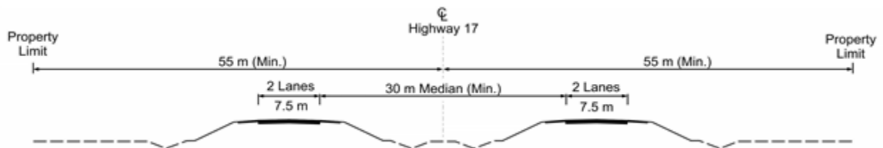
Exhibit 5-9: Typical Cross-Section for Highway 17
